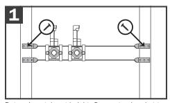
Determine stub out height. Secure top bracket to face of stud bay.
