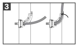
Working from the back of the bracket, insert flexible tube through the nose of the front block then bend tube and capture in place at tail end of elbow.
