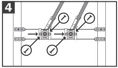
Slide elbow/block assembly to desired stub out location. Insert two screws into each block and tighten. Tightening screws prevents movement of blocks and prevents elbow from swiveling.
