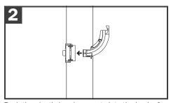
Push the plastic bend supports into the back of each white LockBlock until it clicks in place
