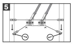
As close as possible to each block, bend the bottom bracket downward. Secure each side of bottom bracket to stud.
